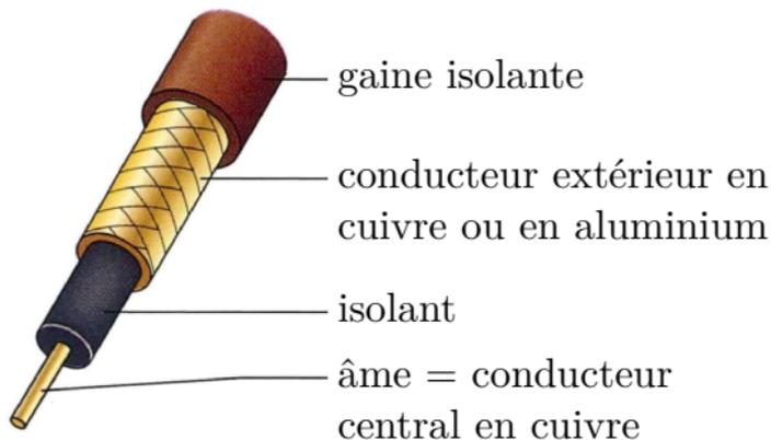
FIG. 2 – Le câble coaxial.
